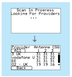
For a reliable 2/3/4G connection it is recommended that for the chosen network (SIM card) used there should be at least two base stations with signal strength (CSQ) of 10 or more.
